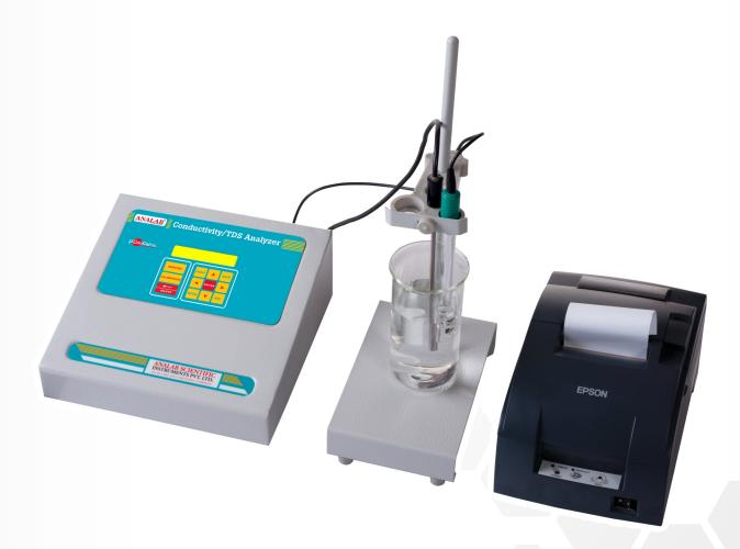
Supplied with Conductivity Cell K = 1.0, Temperature Probe, Electrode Stand consists of Clamp, Base Plate & Rod, Dust Cover, DC Adaptor, Operational & Instruction Manual with SOP, Calibration Test Certificate (Without Traceability Document) and Warranty Card.
