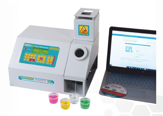
Supplied with Two Filters (Na and K), Inbuilt Air Supply Unit, Atomizer Tube, Sample Beaker (06 Nos.), Gas Lighter, LPG Tube, Power Cord, ANALABsafe software, USB Interface Cable, Operational & Instruction Manual with SOP, Calibration Test Certificate (Without Traceability Document) and Warranty Card.
