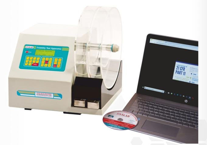
Supplied with Roche Drum - 02 Nos., Drum Holding Knob with rubber bush, Removable Tablet Collecting SS Tray - 02 Nos., Acrylic Tablet Collecting Holder for SS Tray - 02 Nos., Power Cord, ANALABsafe software, USB Interface Cable, Operational & Instruction Manual with SOP, Calibration Test Certificate (Without Traceability Document) and Warranty Card.
