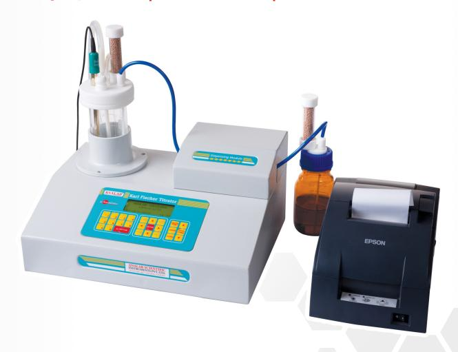
Supplied with 250ml Reaction Vessel, Dual Platinum Combined Electrode, Teflon Paddle, Teflon Assembly, Moisture Trap (02 Nos.), 250ml Amber Reservoir Bottle, Dispensing Tube (02 Nos.), Micro tip (02 Nos.) Teflon Tube for Dispensing Path, Power Cord, Operational & Instruction Manual with SOP, Calibration Test Certificate (Without Traceability Document) and Warranty Card.
